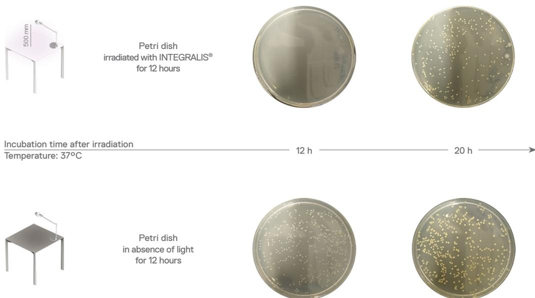
Results of microbiological tests on *Staphylococcus aureus* irradiated with Tolomeo INTEGRALIS®: microbial growth slows down in the hours following irradiation. Scientific findings carried out in collaboration with the Department of Biotechnology and Life Sciences of the University of Insubria.
